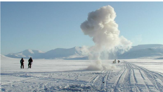
Blasting during seismic survey
